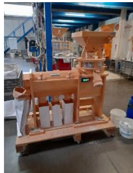
Picture 8. Mélia 30 stone mill (30 cm millstone diameter) manufactured by Alma Pro. Photo credit: ISARA.
